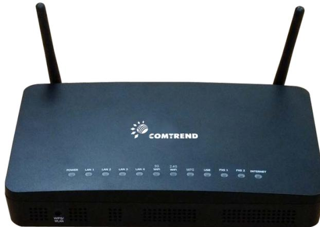
The VG-8061u is an advanced Gigabit Ethernet gateway with 1 Gigabit Ethernet WAN port, 4 Gigabit Ethernet LAN ports, 2 FXS ports, and Wi-Fi. The Wi-Fi not only provides an 802.11n 2T2R 2.4GHz Band which is backward compatible with 802.11b/g but also supports high performance 802.11ac with 3T3R design at 5GHz band.
